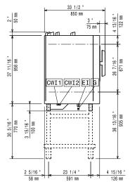
Cold Water inlet 1 (cleaning) = Cold Water Inlet 2 (steam generator) CWI2
